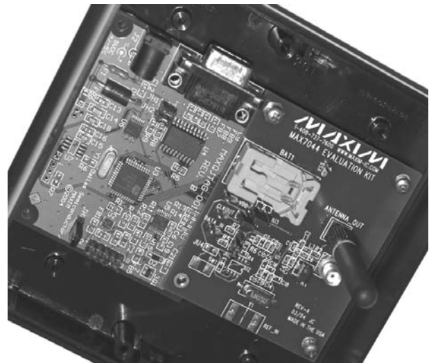
Figure 4. The key-fob transmitter uses two EV kits side by side.
